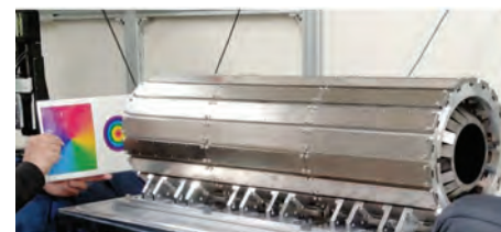
A fully revolutionary metallic neutron focusing ellipsoid mirror
