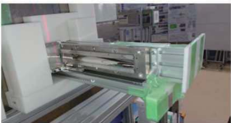
(a) An ellipsoidal neutron focusing mirror on RANS neutron beamline
