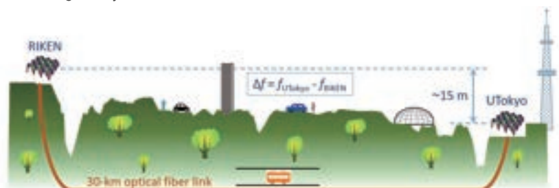
Remote frequency comparison of optical lattice clocks between RIKEN and the University of Tokyo (UTokyo) reveals their different tick rates as predicted by general relativity.
